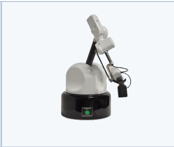
Haption Virtuose: Compact Force-Feedback Devices Desktop 6D
