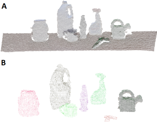
Figure 2: Example of point cloud processing: (A) Original point cloud, (B) Processed point cloud: the main plane in the scene has been removed, and segmentation of the remainder of the cloud has been executed.
