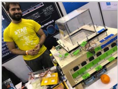
low coast diffusion cloud chamber by Trieste Mini Maker Faire producer Carlo Fonda, with Marco Baruzzo
