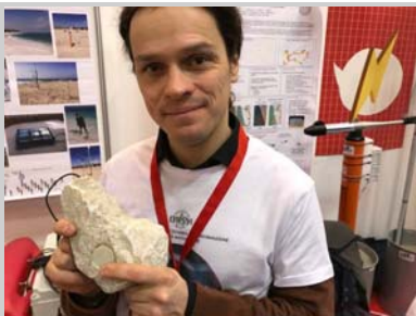
A University research project around measuring erosion with sensors (including this one embedded in rock) to measure rock movement and sand displacement
