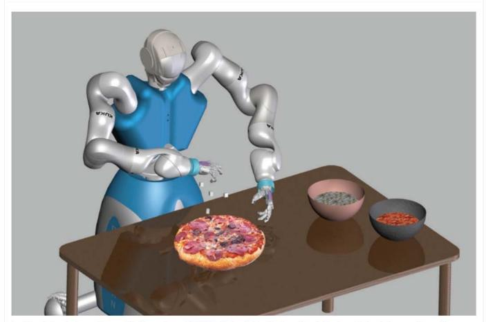
In this video lecture, Bruno Siciliano from PRISMA Lab at the University of Naples, Italy, takes us through a new project in robotic dynamic manipulation, called RoDyMan. Centered on the task of making a pizza, the project aims to solve key problems related to robot gripping: localisation of the object while it is moving, motion and manipulation of the object, and control of the overall robotic system.
