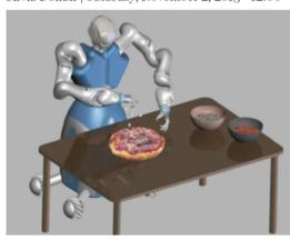
A robot that can make pizza: roll out the dough, add toppings, put it in the oven and rotate it when necessary.
