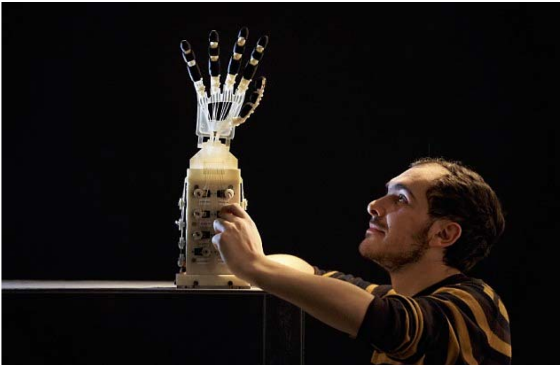
Robotics student Gildo Andreoni works on a Dexmart robotic hand built at the University of Bologna. Dexmart's hands are 'smart' enough to make cups of coffee and pick up clothes from the floor
