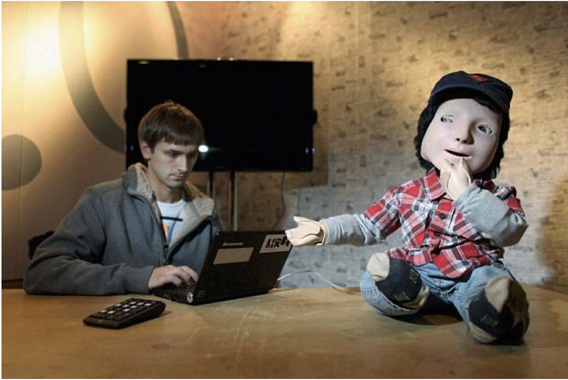
Robotics PhD student Luke Wood works on Kaspar, a robot built at the University of Hertfordshire to help autistic children interact with people
