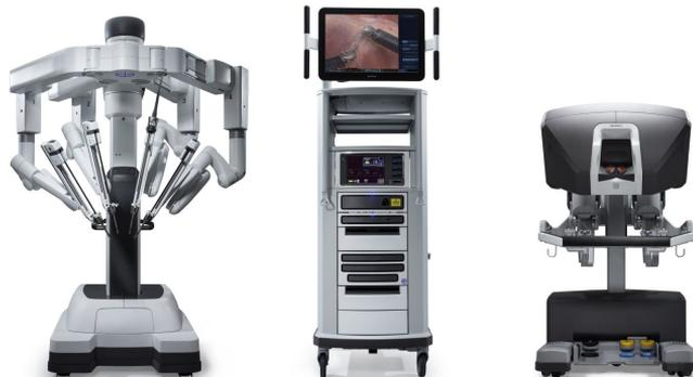
**Figure 1.3.** The da Vinci<sup>TM</sup> Xi robotic platform.
