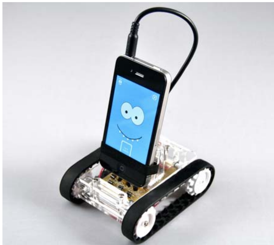
Romotive, a Seattle start-up, created a tracked mobile robot powered by a smartphone. Photo: Romotive
