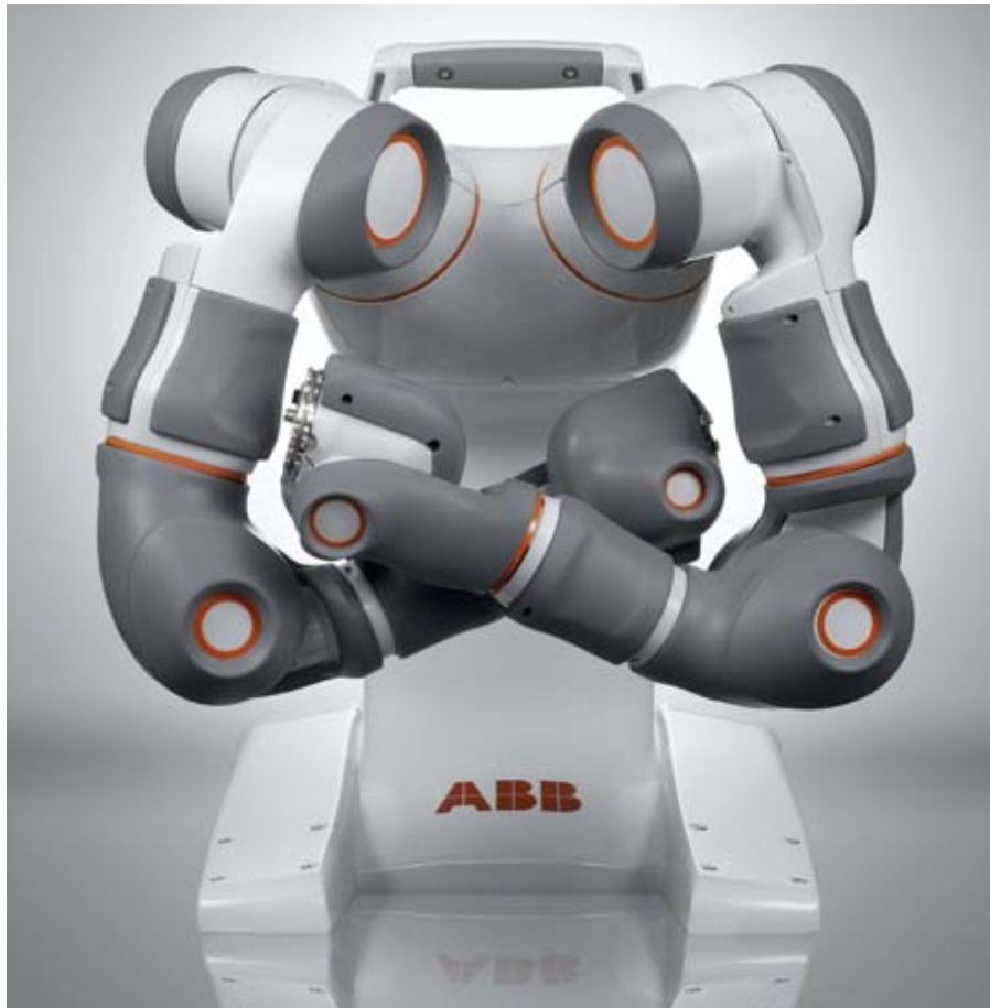
The ABB FRIDA concept is a 14-axis dual arm robot designed for working alongside human workers in manufacturing environments. Photo: ABB
