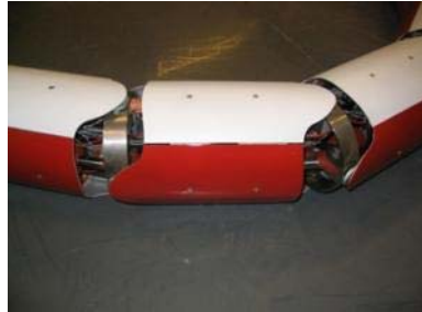
The Anna Konda is a snake-like robot that can also avoid obstacles and put out fires. (Credit: Image courtesy of ICT Results)
